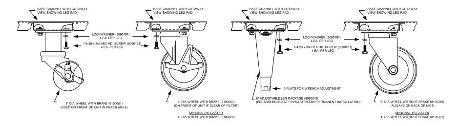
NOTE: WHETHER INTALLING CASTERS OR LEGS, ALWAYS USE FOUR EACH 1/4-20 X 3/4 HEX HEAD SCREWS (8090131) WITH FOUR EACH LOCKWASHERS (8090191) FOR EACH CASTER OR LEG ASSEMBLY, AND TORQUE EACH SCREW TO 50 INCH-POUNDS MINIMUM. SEE DIAGRAMS ABOVE FOR PROPER LOCATION OF LOCKWASHERS.
